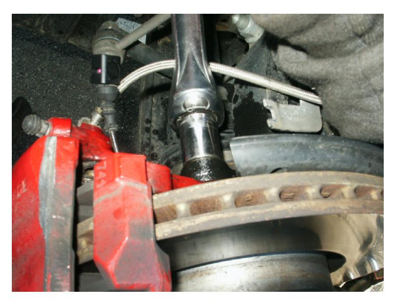
Step 7: Slide the caliper off the rotor, and support so there's no stress on the brake line (I usually wheel the jack over and use it to hold the brake caliper up while I work).
