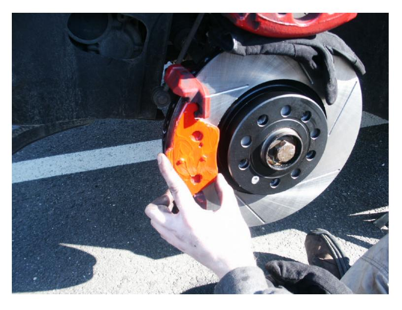
Step 20: Slide the caliper back onto the caliper carrier. Re-secure with the caliper carrier pins. Be sure to replace the black plastic covers on the caliper carrier pins, and reconnect the wear sensor if your new pads have one.
